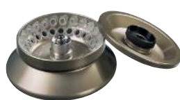
Angle rotor, 24-place Cat. No. 02428 n = 15,000 \text{ min}^{-1} , max RCF 21,382 incl. bioseal lid
