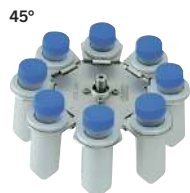
Swing-out rotor, 8-place, n = 5,000 \text{ min}^{-1} , RCF 3,857, for 8 x 50/15 ml, stainless steel, with suspensions, aluminium.
