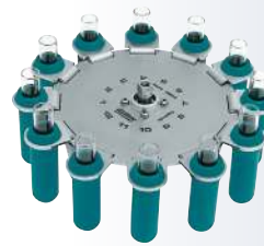
Swing-out rotor, 12-place, for 12 x 15 ml n = 4,000 \text{ min}^{-1} , RCF 2,683, Stainless steel, with suspensions No. 01621, PA, fiberglass rein- forced.
