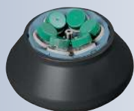
Angle rotor, Cat. No. 01556 6-place, n = 9,000 \text{ min}^{-1} , max. RCF 10,595
