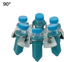
Swing-out rotor, 6-place, for 6 x 50/15 ml Falcon tubes n = 4,000 \text{ min}^{-1} , RCF 2,701, Stainless steel, with suspensions, PA, fiberglass reinforced.
