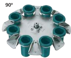
Swing-out rotor, 8-place, for 8 x 15 ml, n = 4,000 \text{ min}^{-1} , RCF 2,415 Stainless steel, with suspensions No. 01644, PA, fib- reglass reinforced.
