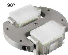
Swing-out rotor, 2-place, n = 4,000 \text{ min}^{-1} , RCF 2,218 for microtitre plates, aluminium, coated, with suspensions No. 01453-A, stainless steel.
